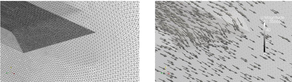
*Mesh (left) and Flow Field (right) of non-serrated flat plate trailing edge*
