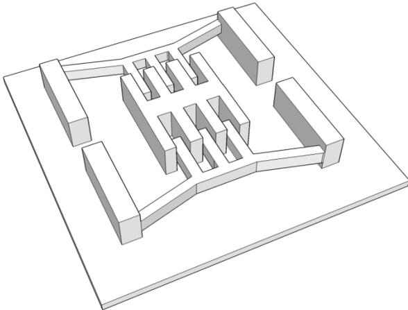
*The proposed MEMS-based capacitive strain sensor*
