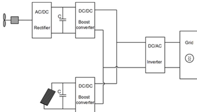
*Schematic diagram for the hybrid PV-Wind system*
