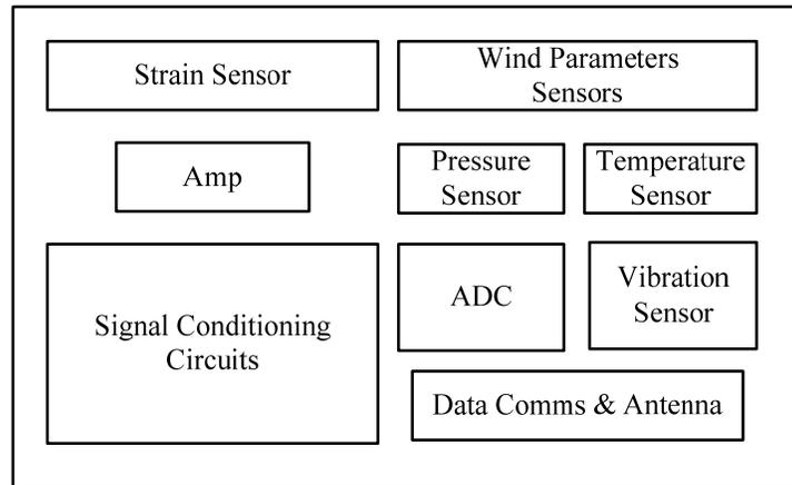
*Proposed integrated smart sensor for wind turbine blades*
