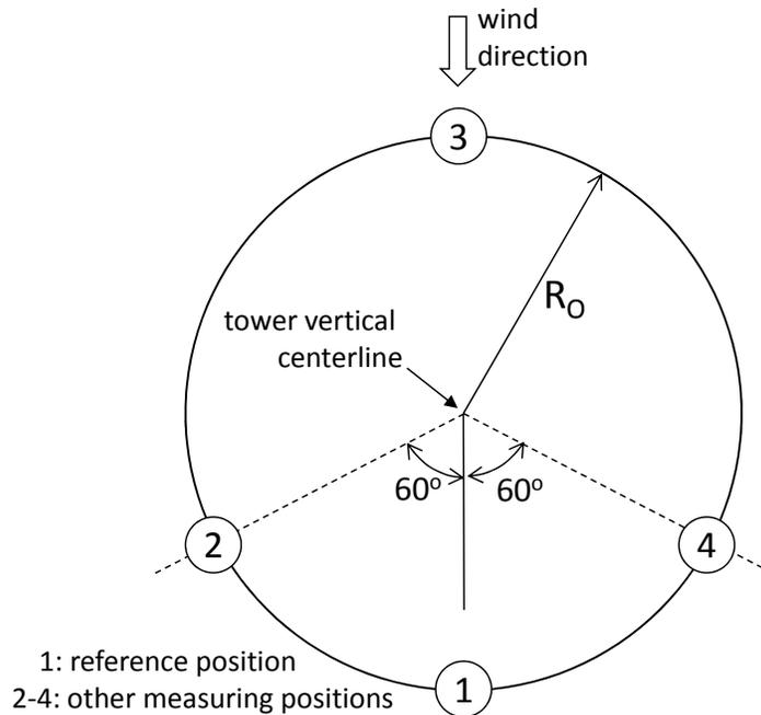
*Typical microphone positions for the noise measurements (after ICE 61400-11: 2002)*
