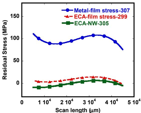
Figure 5a: Residual stress in silicon wafers with screenprinted metal and ECA layers.
