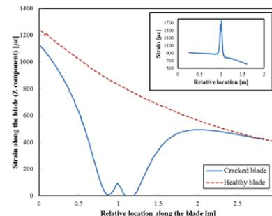
Figure 2d. Sudden change of strain magnitude is detectable near damage locations
