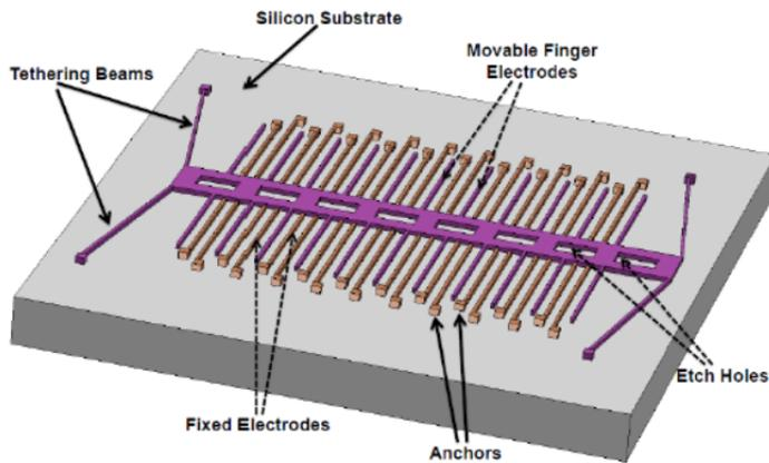
Figure 3a: Differential capacitive strain sensor with four mechanical amplifying beams
