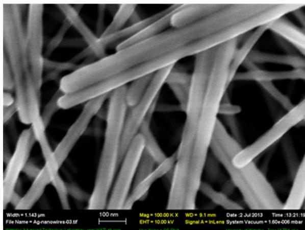
Figure 5b: Scanning electron micrograph of Ag nanowires used to develop the ECA material (scale bar = 100nm)
