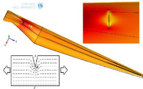
Figure 2b. Damaged blade's strain field distribution
