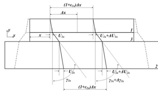
Figure 3c: Displacement equilibrium diagram of the investigated adhesive bonded structure
