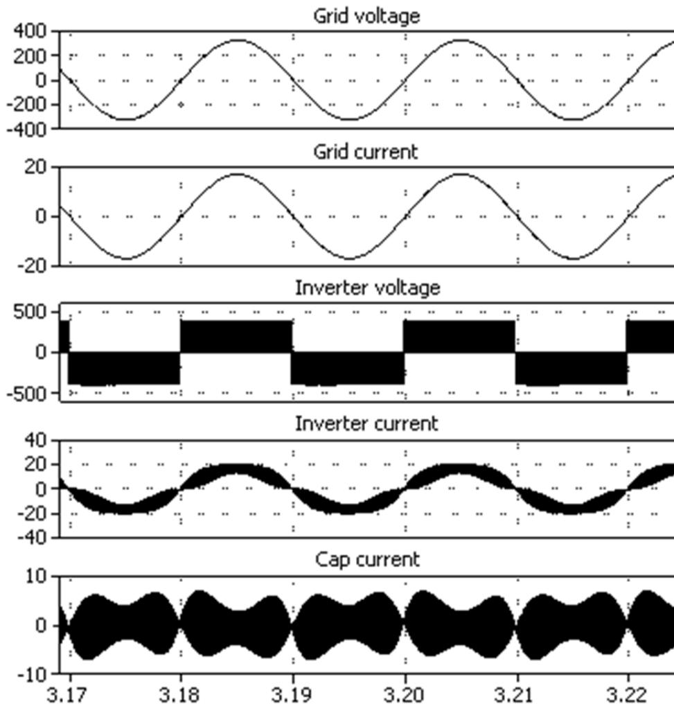
Figure 4: Waveforms of the grid and inverter voltage and current and, current passing through LCL filter capacitor
