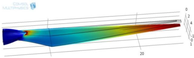
Figure 2a. Finite element method simulation model of wind turbine blade under various load conditions.
