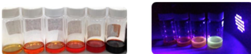
Figure 4: Solutions containing the synthesized CIS QDs of different sizes extracted at different growth times before (left,) and after (right), illumination with ultraviolet light.
